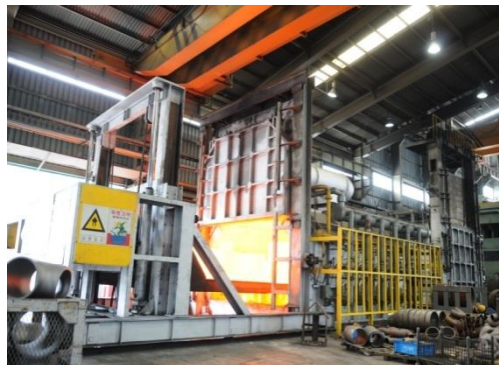
Heat Treatment Furnace For Fitting
