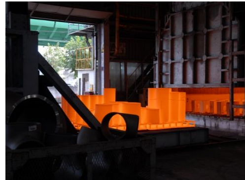
Solution Heat Treatment Furnace
