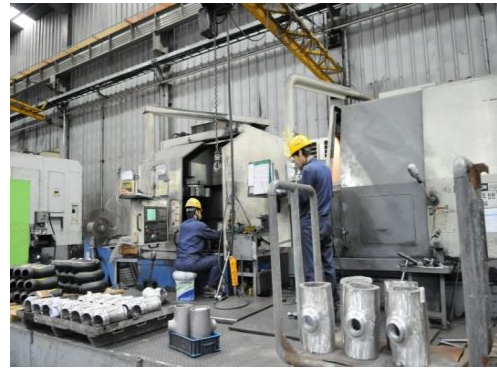
CNC Boring Machine
