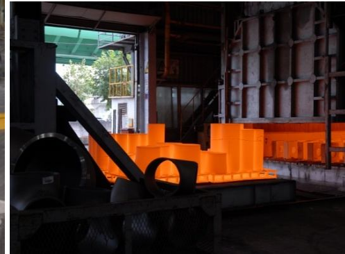
Solution Heat Treatment Furnace
