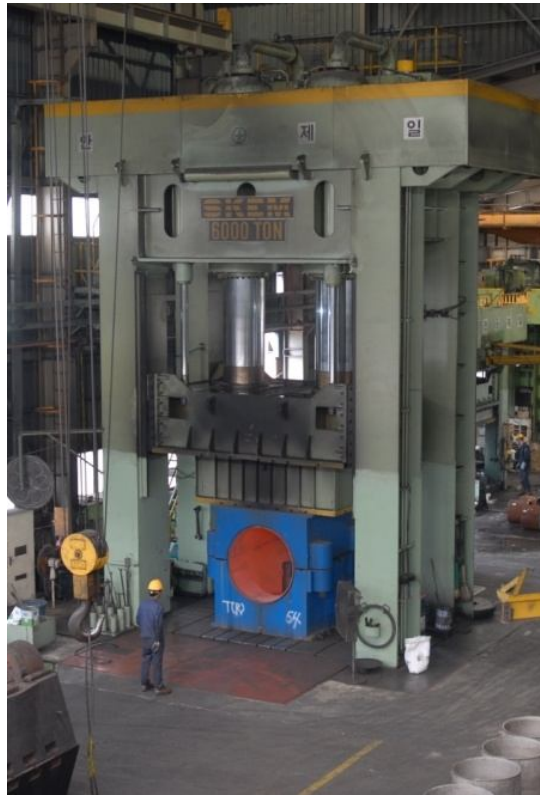
5,000 Ton Hydraulic Press
